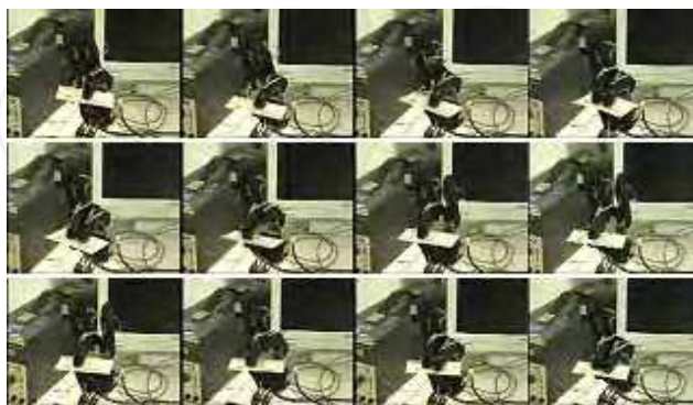
Fig. 14. Snapshots of the robot hand handling a business card using two or three fingers.
