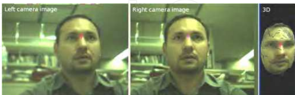
Fig. 8. Screen capture of the left and right camera images, and OpenGL plot of texture mapped 3D face reconstructed by the stereo algorithm.
