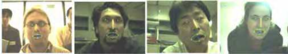
Fig. 6. Screen capture of tracked outer lip contours for various skin tone colors and different lighting conditions.
