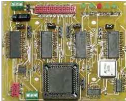
Fig. 21. The prototype custom embedded real-time controller. The board has dimensions of 69 \times 85mm^2 .
