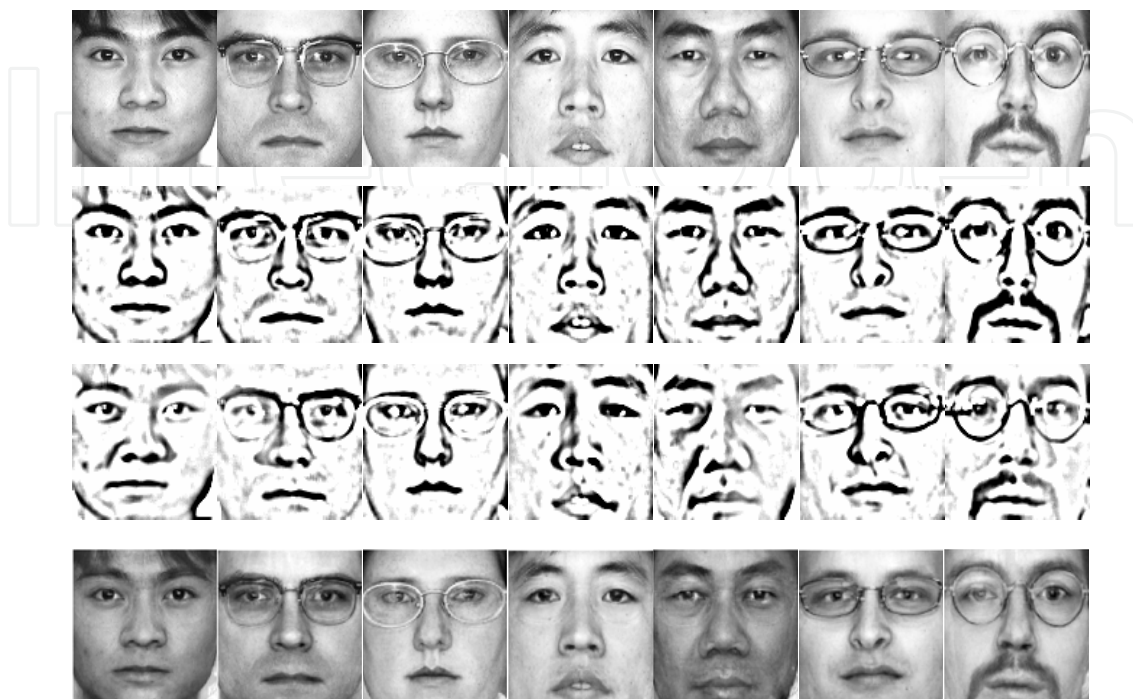
Figure 11. Examples from CMU PIE database (first row) example face images in training database (second row) corresponding sketch images with respect to the first row (third row) given probe sketch images (fourth row) reconstructed (hallucinated) face images based on the hybrid-subspace approach
