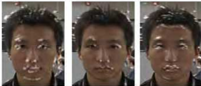
Figure 8. Intermediate output from MCoNN (1):input image, (2) output example from FD1, (3) intermediate outputs from encircled modules of FD2 in Figure 7
