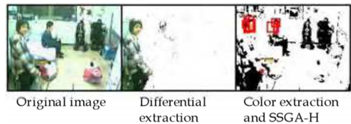
Figure 7. Human detection results from the ceiling camera of the environmental system by SSGA-H
