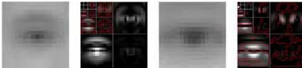
Figure 6. From left to right: the mean eye pattern, its wavelet decomposition and the selected features (red contour) of the two eye patterns. High intensities correspond to strong edges, low intensities indicate uniform regions
