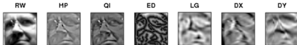
Figure 11. Examples of the evaluated face representations: raw grey scale input (RW), high-pass filtered data (HP), the Quotient Image (QI), distance-transformed edge map (ED), Laplacian-of-Gaussian filtered data (LG) and the two principal axis derivatives (DX and DY)
