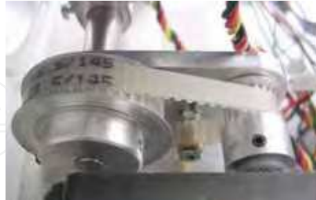
Figure 3. Transmission with a 2.5:1 gear ratio; an adjustable tensile roller holds the belt tight As mention earlier, power to drive the motors is a most relevant issue. Servos absorb high currents, especially at start-up. Two ion-lithium batteries were installed and the system counts with a 7.2 V/9600 mAh pack, with maximal sustained current specified by the vendor at more than 19A. Each one of the two batteries weights circa 176 g. Proper fusing and charge monitoring were also implemented. Figure 4 shows the selected batteries and their location on the robot.
