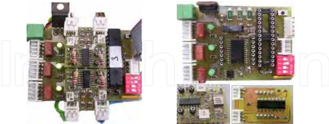
Figure 11. Complete Slave Unit (left); base board and two cases of piggy-back boards (right)
