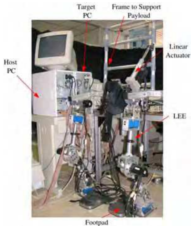
Figure 24. Set-up of developed control system
