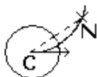
Fig. 1. A robot currently at location C moves along a clothoidal arc to reach position N. The aspiring orientation is computed as mentioned in premise a in text. The heading at C is indicated by the arrow
