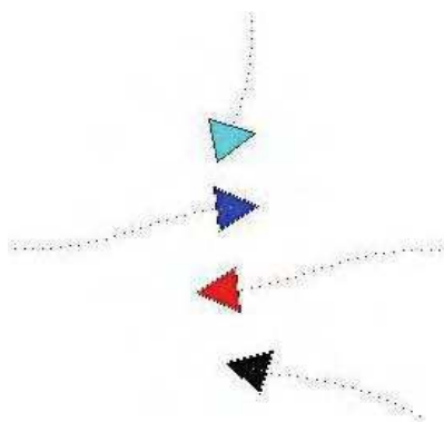
Fig. 15c. In order to minimize the optimization function robots black and cyan change their directions and avoid collision.
