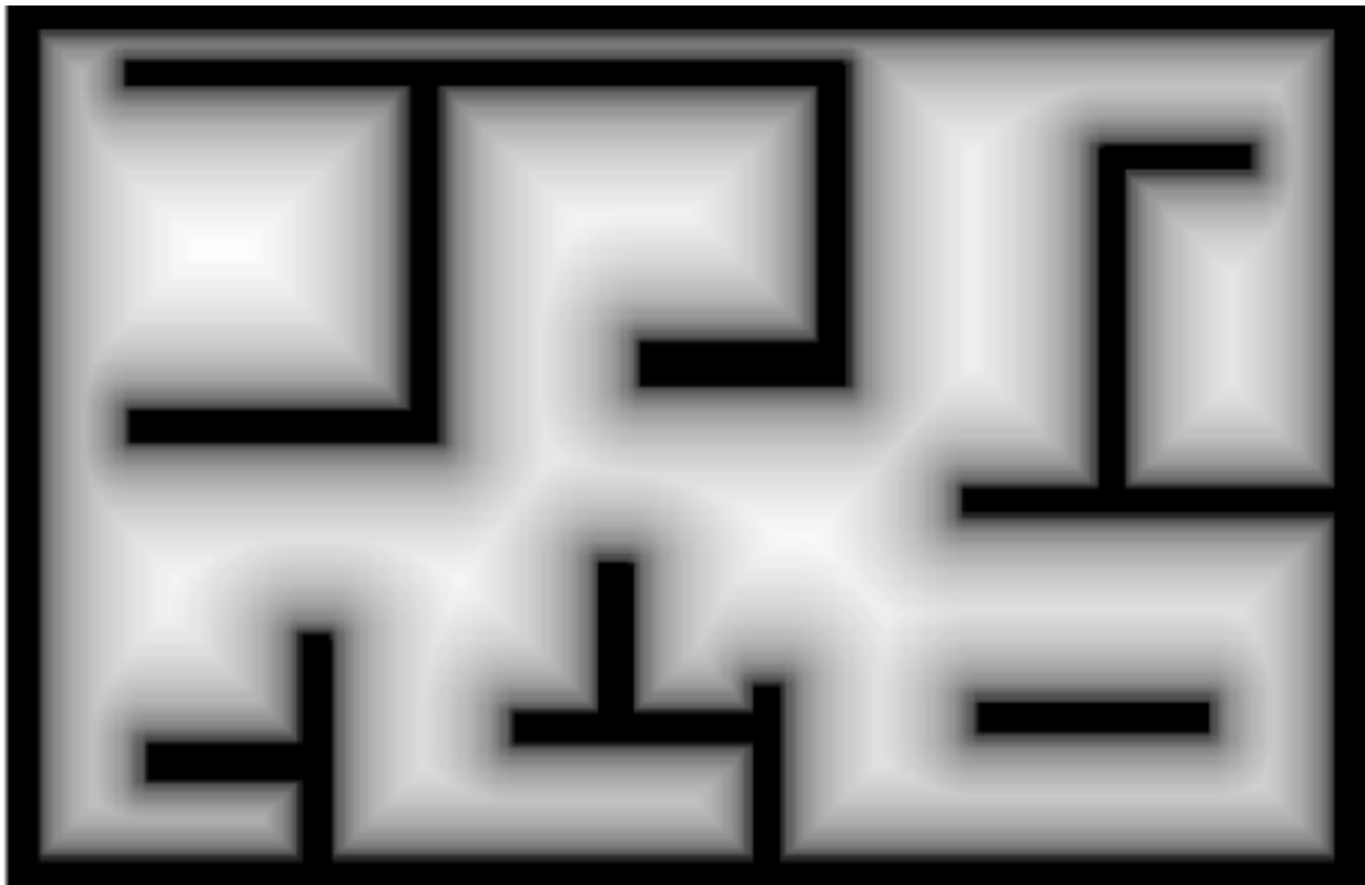
Fig. 4. Potential of the Extended Voronoi Transform.
