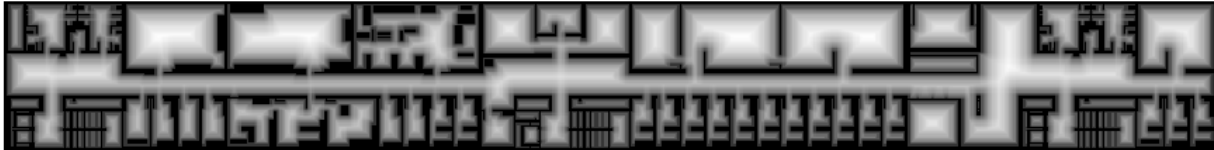
Fig. 10. Extended Voronoi transform of the UC3M Robotics Lab plan
