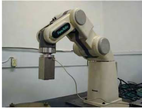
Fig. 4. Robot equipped with the three-axis tactile sensor.
