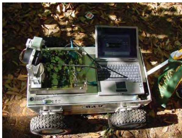
Fig. 2. Mobile robotic platform with computer-controlled scanner holding ultrasound transducer.
