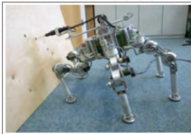
Fig. 3.7. Robot "Katharina" by drilling.
