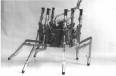
(f) Six-legged robot Silex (15 kg). Free University, Brussels.
