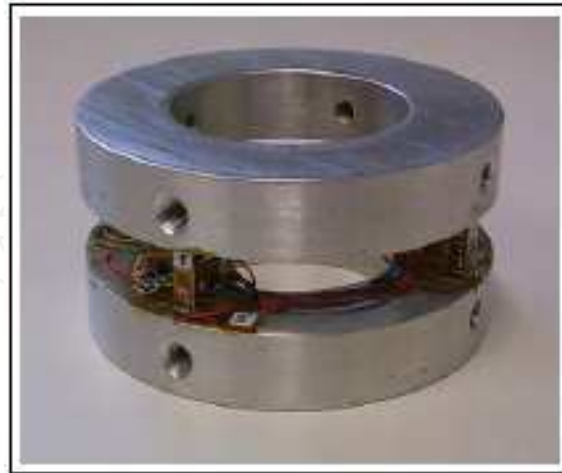
Fig. 3.6. Three-component force sensor for high loading.
