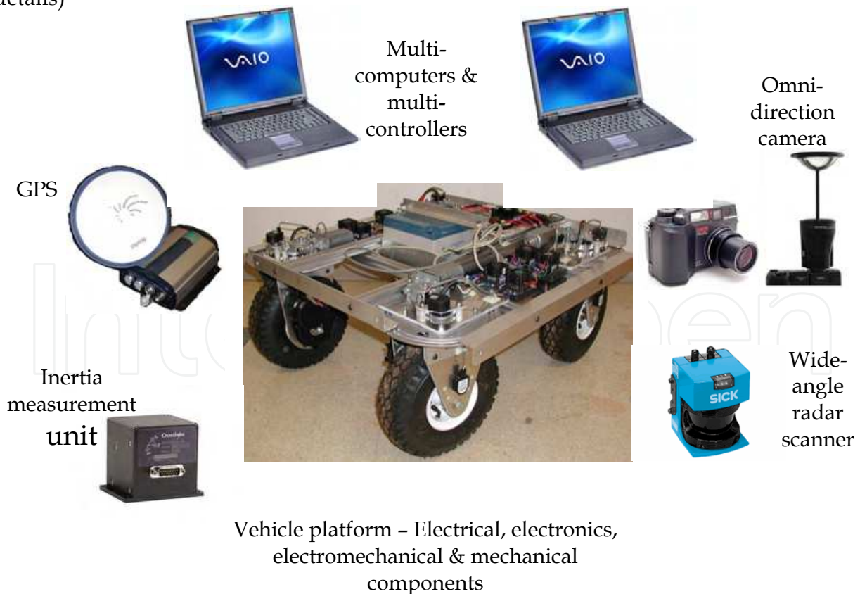
Fig. 2. Typical technology make-up of an IGVC vehicle.
