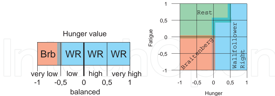
Fig. 3. The quantised internal values (e.g. Hunger and Fatigue) are quantised into four segments; each segment is assigned a behaviour primitive (action selection matrix).
