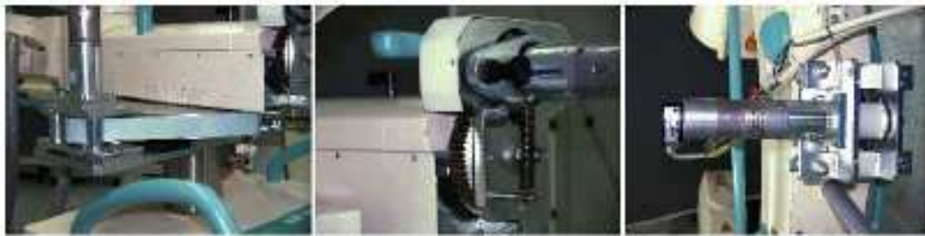
Fig. 5. Joints two, four and five with external drives, gears and encoders.
