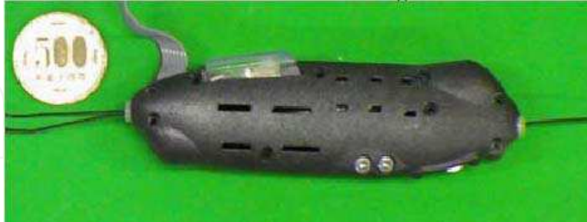
Fig. 2. A newly-developed, sensors-integrated muscle unit.
