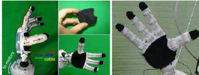
Fig. 11. Soft and fleshy tactile sensor using conductive rubber foam.
