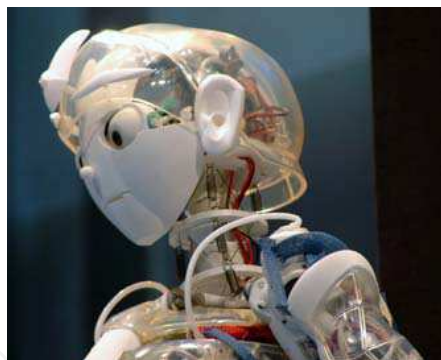
Fig. 10. Muscle-driven head for multi-modal communication.
