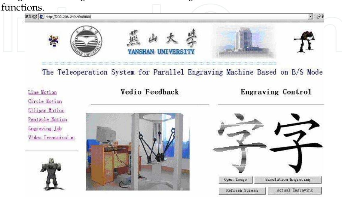
Figure 21. The interface of teleoperation system for engraving
