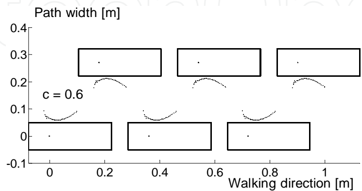
Figure 27. Mechanism footprints of decelerated motion for c = 0.6 . No compensation applied.
