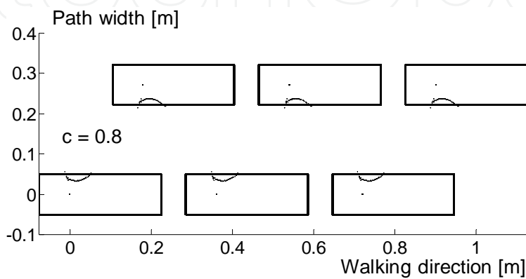
Figure 25. Mechanism footprints of decelerated motion for c = 0.8 . No compensation applied.
