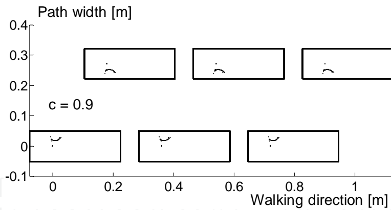
Figure 24. Mechanism footprints of decelerated motion for c = 0.9 . No compensation applied.
