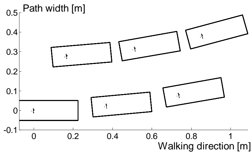
Figure 4. Mechanism footprints when \alpha is 5°. No compensation applied
