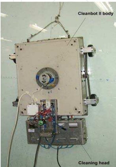
Figure 2.2 Climbing robot “Cleanbot II”
