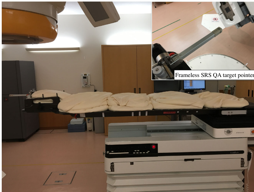
FIG. 3. The aspect of the frameless SRS QA target pointer on the weighted couch with a phantom study.
