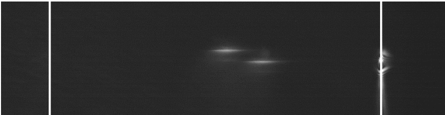
Figure 2.4. Image of two filaments at different on-axis positions generated in the bulk of a 5-mm thick fused silica sample (white bars denote the limits of the fused silica sample).
