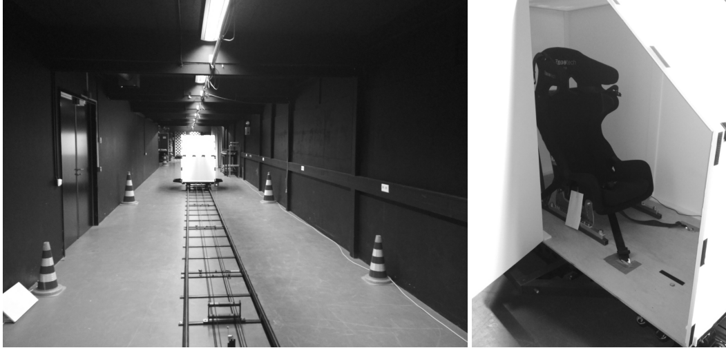
Fig. 1a: The 40 m track with the cabin. Only 9 meter peak-to-peak motion was used for the present purpose. Fig. 1b: The cabin interior. The cabin prevented visual and somatosensory (via airflow) information from giving participants information on the occurring motion.
