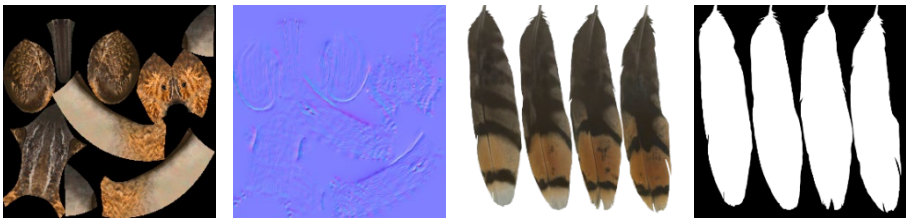
Fig. 6. Diffuse and normal map for the 3D model of the Snipe. Diffuse and opacity map for its feathers.
