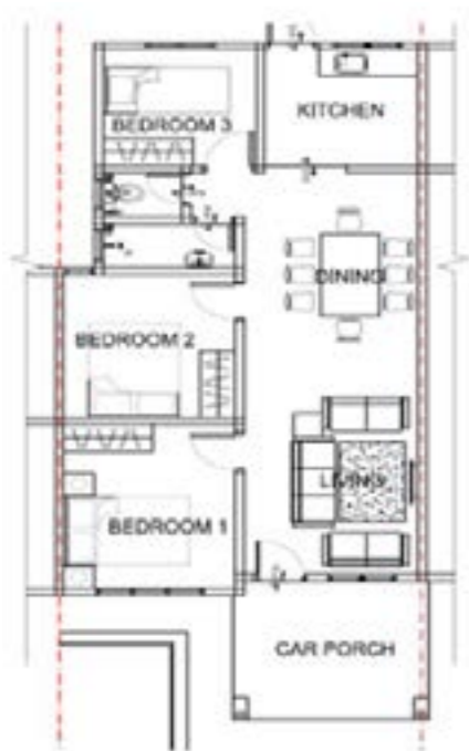
Figure 2 : Typical layout of a low-cost house
