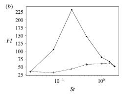
FIGURE 3. (Colour online) (a) The p.d.f.s of the bubble acceleration normalized by its root-mean-square value in black for St = 0.02, 0.074, 0.20, 0.45, 1.01, 1.55 and 2.07 (shifted upward by two decades from each other for clarity, respectively) and comparison with the p.d.f.s of the acceleration of fluid tracers in red. (b) Flatness of the bubble acceleration ( $\bullet$ ) and of the fluid acceleration at the bubble position (+) against St from our DNS.
