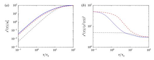
FIGURE 11. (Colour online) (a) Evolution of the second-order Lagrangian structure function with the time lag. (b) Evolution of the flatness of the Lagrangian velocity increments with the time lag. Comparison between the DNS (solid blue line), the Standard LES (black dot-dashed lines) and LES with the proposed model (dashed red lines). For both figures, for St = 0.02, the mesh size for the LES is  $64^3$ .
