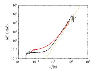
FIGURE 12. (Colour online) Variance of the total bubble acceleration  $a_b = \overline{a}_b + a_*$  conditioned on the stochastic value of the dissipation rate  $\varepsilon_*$  obtained from the LES with the stochastic model (black line) and comparison with the bubble acceleration variance conditioned on the local dissipation rate obtained from the DNS (red line), with St = 0.02 and a mesh size of  $48^3$  for the LES.
