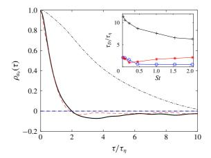
FIGURE 10. (Colour online) Autocorrelation of the bubble acceleration for St = 0.07. The DNS is a solid black line, LES with model for  $64^3$  is a dashed red line and LES without model for  $64^3$  is a dot-dashed black line. The inset is the evolution of the corresponding integral time scale normalized by the Kolmogorov time with the Stokes number. The DNS are circles, LES with the proposed model are stars, LES without model are crosses. The mesh size for the LES is  $64^3$ .
