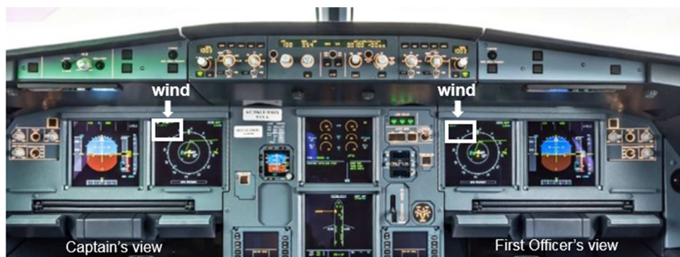
Figure 2. An example of the reference image with the area of interest (wind). Analyses were focused on the decision relevant item in the cockpit.
