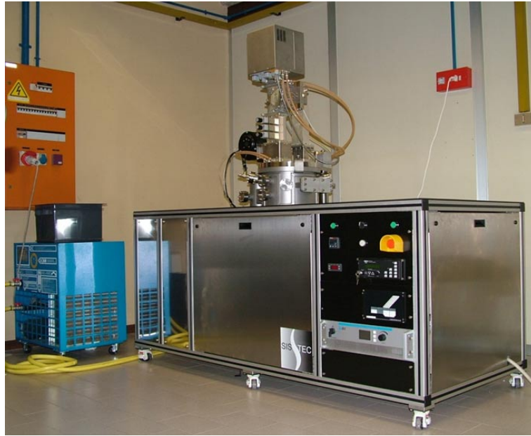
Fig. 1. – Scheme of the MW/RF-PECVD apparatus.
