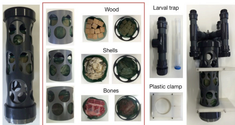
Fig. 5.5 LO 3 CATED modular sampling device. From left to right: settlement frame [14 cm Ø; 55 cm height] enclosing containers [12.5 cm Ø; 13 cm height] with experimental biogenic substrates; larval traps consisting of three stacked 50 ml Falcon tubes, which are inserted inside a PVC tube and can be attached on top of the settlement frame in a cross arrangement. The complete device can be fixed to the mooring line with plastic clamps.
