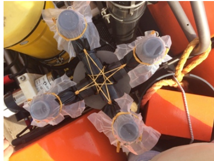
Fig. 5.7 Larval traps covered with parafilm secured with rubber bands and magnesium links.
