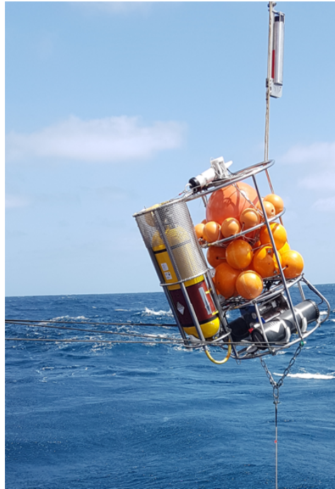
Fig. 5.8 Underwater winch during deployment at Senghor Seamount.
