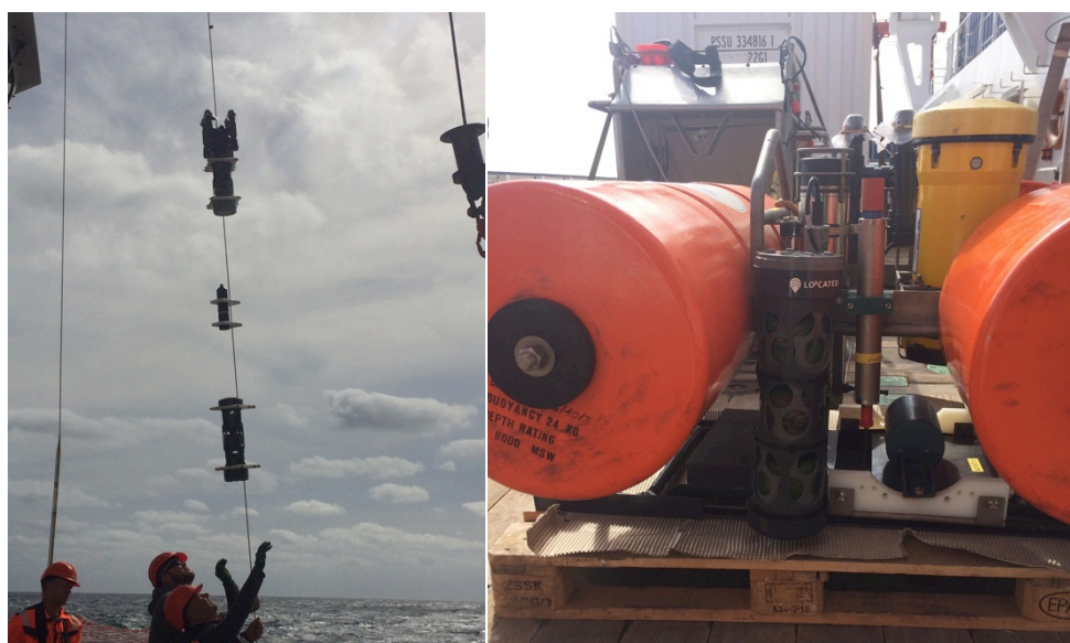
Fig. 5.6 LO 3 CATED sampling devices attached to mooring cable (left) and lander (right) for deployment at Senghor seamount.
