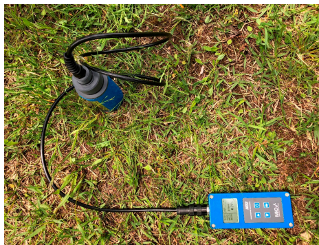
Figure 2. Time-domain reflectometry (TDR) measurements of the soil moisture for the estimation of the subsurface velocity in the site.
