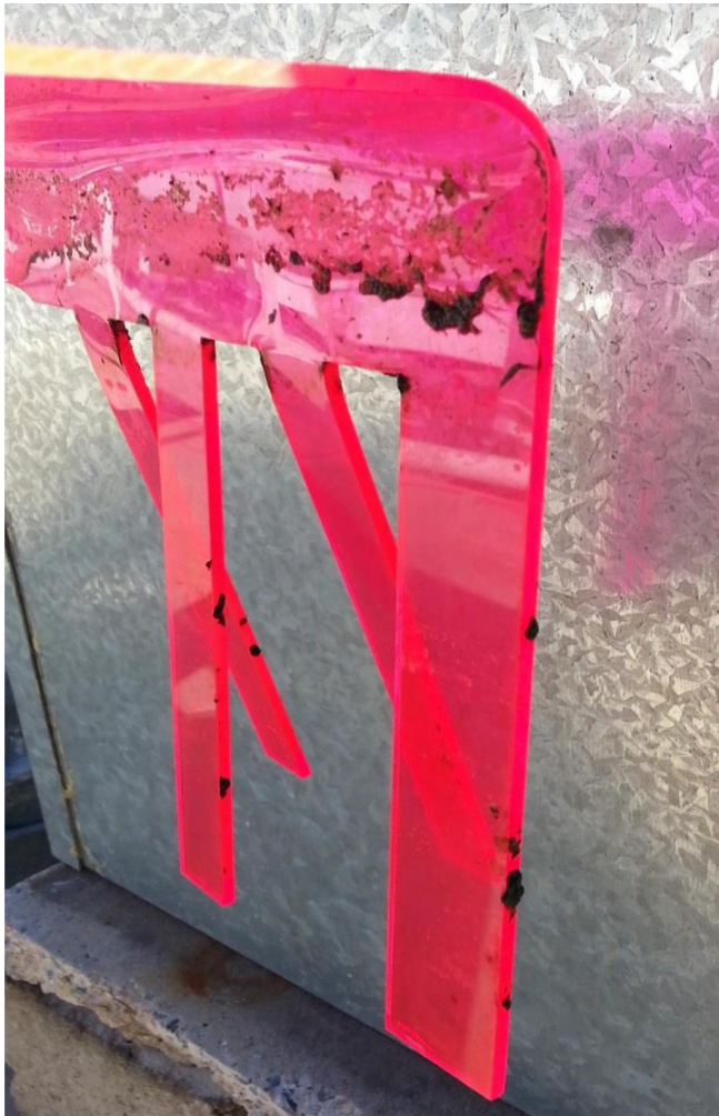
Figure 3-6. Arthrospira platensis biofouling on a luminescent solar concentrator during 75 days of the cultivation period.
