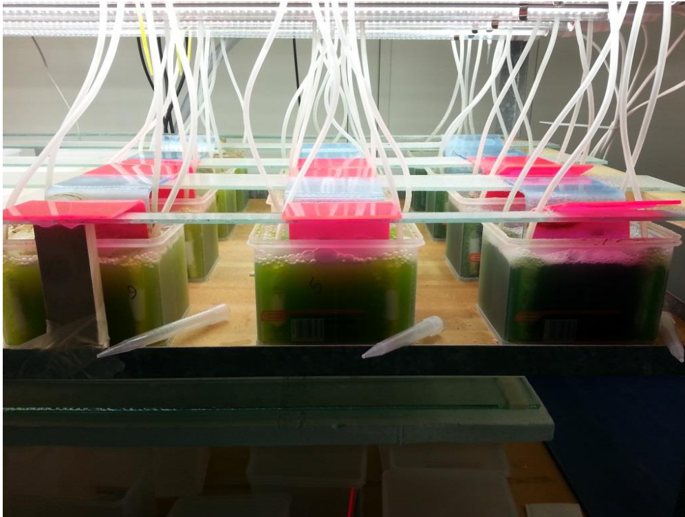
Figure 2-1. Structural view of photobioreactors equipped with red and blue luminescent solar concentrators with the culture volume of 1 L for each reactor. In this study, four reactors were used as with a) red & blue LSCs, b) two red LSCs, c) two blue LSCs and d) control with no LSCs for each species of Arthrospira platensis , Scenedesmus sp. and Chlorella sp. In a batch mode. The cultures were mixed by aeration.
