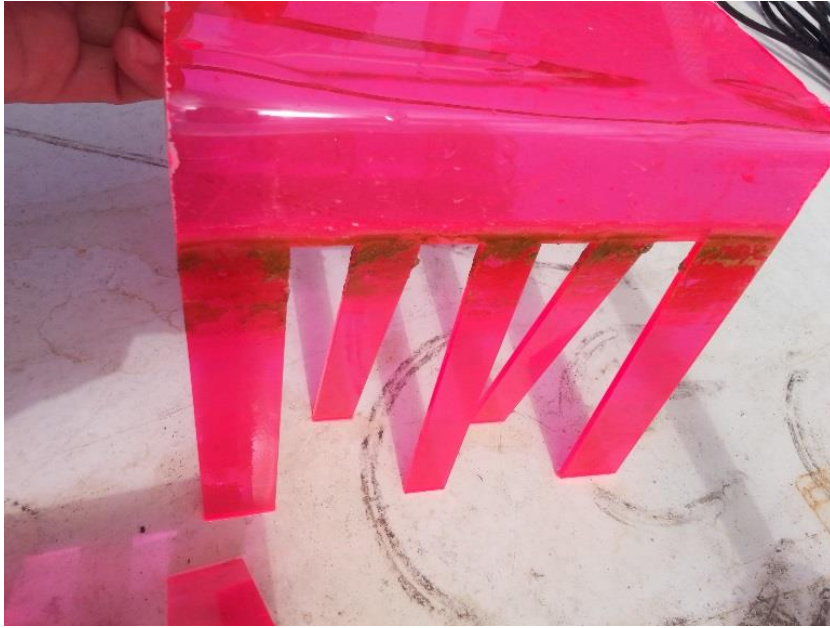
Figure 4-6. Scenedesmus sp. biofouling on a luminescent solar concentrator during 15 days of the cultivation period.
