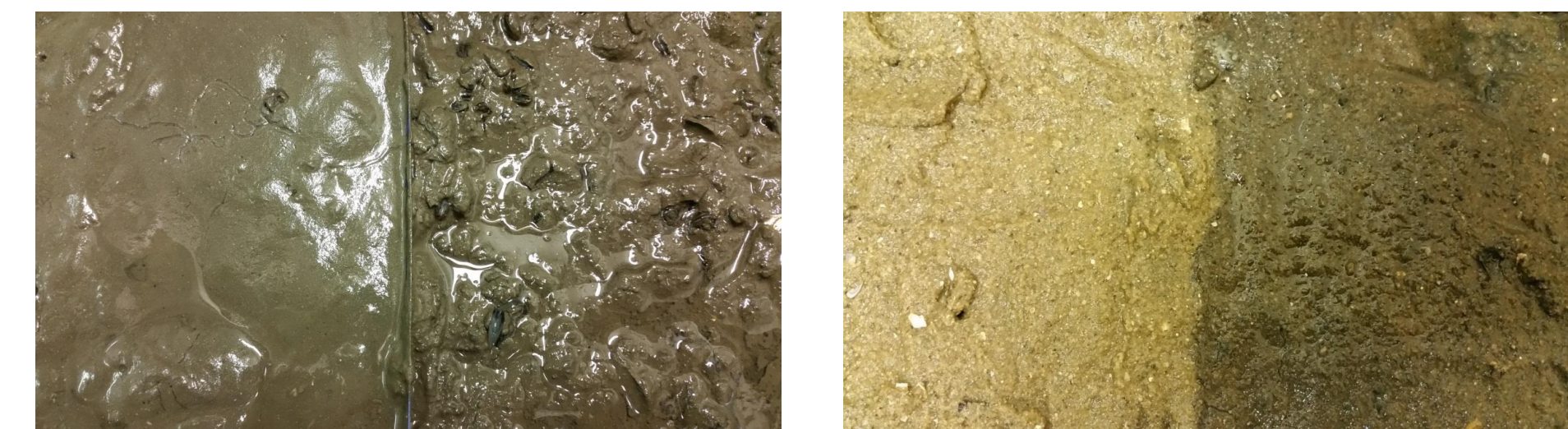
Fig. 6: Photos looking into the experimental tanks containing sediment from (a) deep and (b) shallow waters. Sediment from lower estuary on left hand side.
