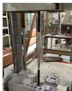
Figure 2: Tensile testing of GFRP bars
