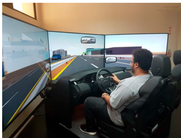
Figure 1. Installed driving simulator at Qatar University (Range Rover Evoque)
