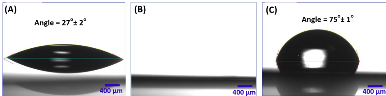
Figure 4.1 Contact angle measurements for treated silicon substrates. (A) Bare silicon, (B) Plasma-cleaned silicon, (C) Spin-coated silicon with PGMA- b -PVDMA (after annealing and sonication in chloroform).
