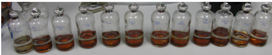
Figure 5.2. Insoluble iron(III) reduction assay for testing functionality of Shewanella cytochromes in E. coli .
