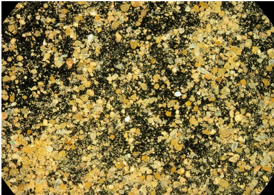
Figure 4-8 Light Microscope Image of Siliceous Gravel (A5) Smaller than 0.15 mm (Passing Sieve #100)
