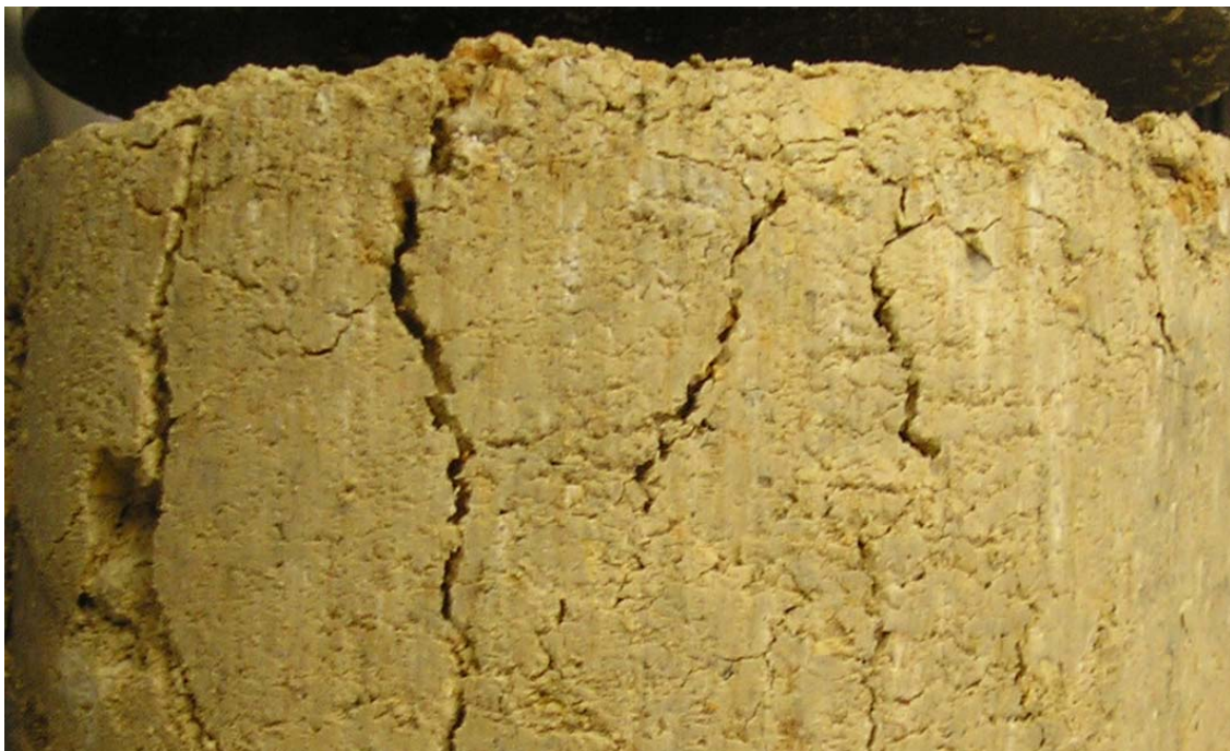
Figure 4-4 Shear Banding in 2 Percent Cement Stabilized High Fines System V3
