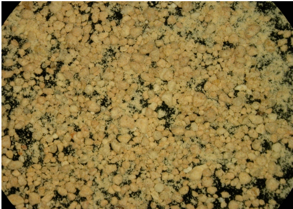
Figure 4-14 Light Microscope Image of Limestone (A2) Smaller than 0.15 mm (Passing Sieve #100)
