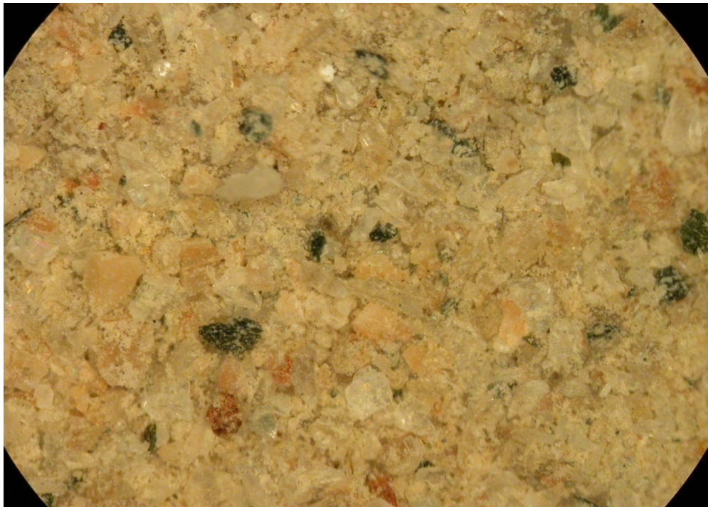
Figure 4-6 Light Microscope Image of Granite Materials (A8) Smaller than 0.15 mm (Passing Sieve #100)
