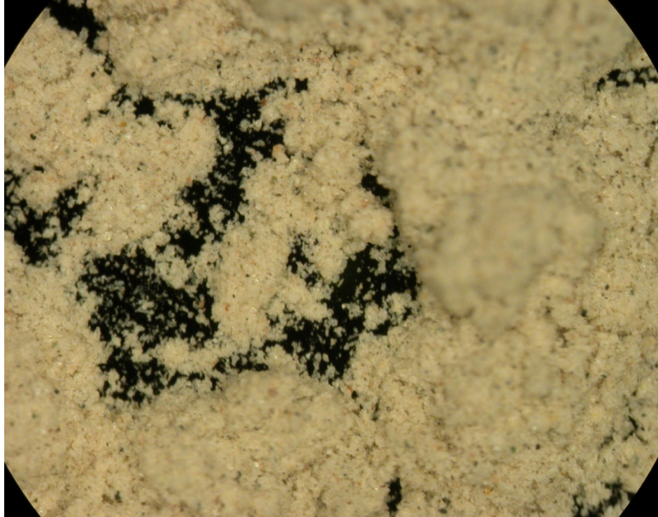
Figure 4-7 Light Microscope Image of Granite Materials (A8) Smaller than 0.075 mm (Passing Sieve #200)
