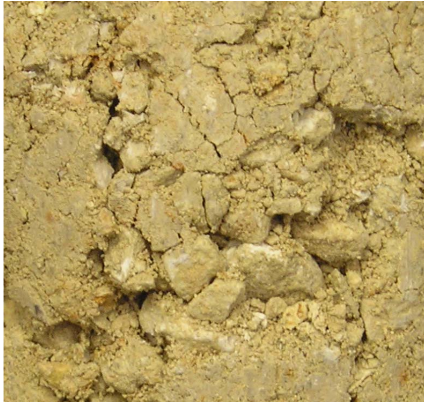
Figure 4-5 Degradation of Particles for Coarse Gradation V1 under Wet Conditions
