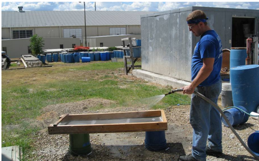
Figure 7.2: Washing Microfines out of Manufactured Sands.
