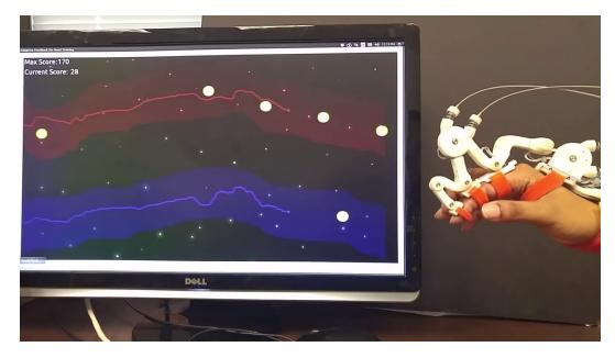
Figure 4.2: The index finger exoskeleton module and the graphical user interface presented to the subject for the motor learning study.
