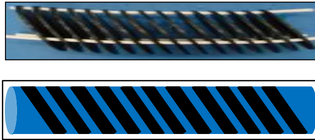
Figure 3.17: (a) A 2-foot-long, 4-inch-diameter synthetic whole core comprising 0.25-inch TIVAR elliptical discs separated by 0.75 inches and oriented at 45°-dip. (b) Schematic of such a whole core.
