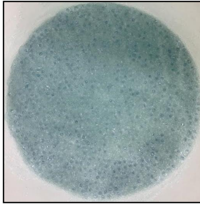
Figure 3.15: Top view of 4-inch-diameter brine-filled glass-bead pack identifying vuggy isotropic whole core. Uniformly distributed 6-mm glass beads identify non-conductive vugs, and the remaining brine-filled volume made of 1.15-mm-diameter glass beads identifies the fluid-saturated porous matrix.
