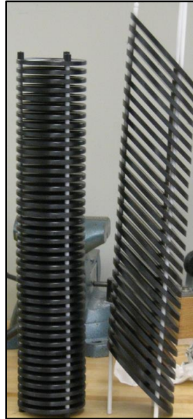
Figure 3.4: Frameworks of two synthetic bilaminar whole core samples of 0°-dip (left) and 45°-dip (right), respectively.
