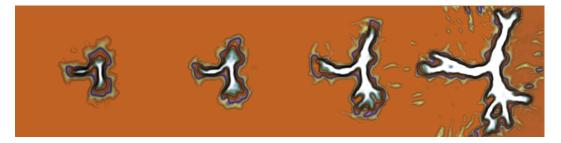
Figure 6.1: Evolution of two pressurized fractures: first joining, then nonplanar growth and finally branching in heterogeneous porous media.
