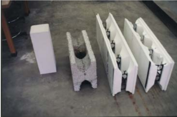
Figure 1.2. Residential Concrete Building Systems. Left to Right: Hebel Block, ICF, and Polystyrene.
