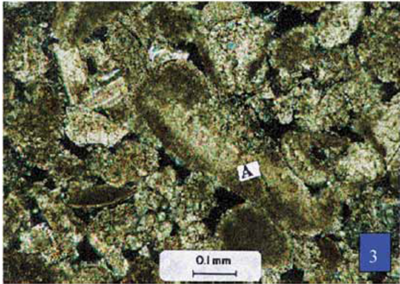
Figure B.3. An Elongated Particle (A) with a High Aspect Ratio of 8:1 (Source Number 1).
