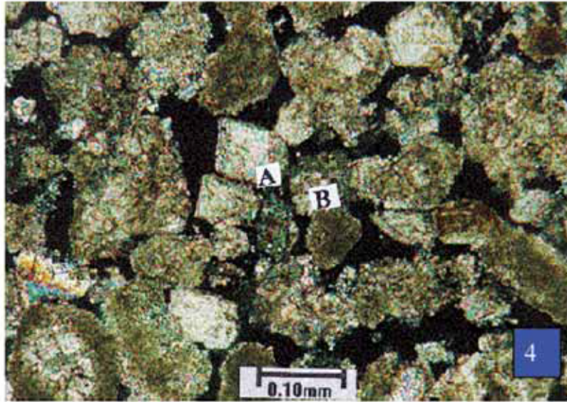
Figure B.4. Distribution of Dolomite Rhombs (A) and Subrounded Calcite Crystals (B) (Source Number 1).
