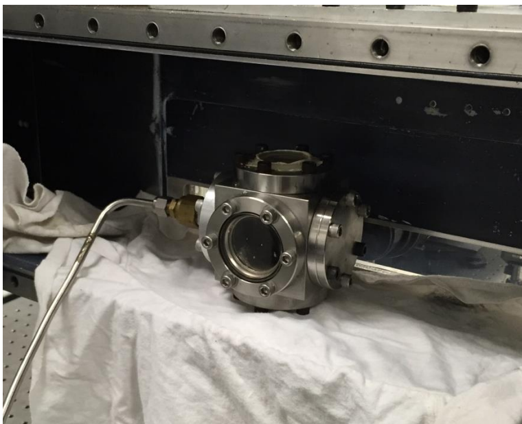
Figure 3.4: Photograph of the room temperature, pressure-controlled reference cell inside the Mach 5 test section.
