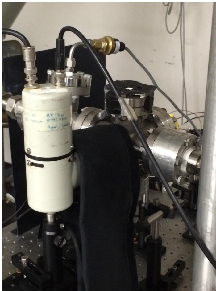
Figure 2.2: Photograph of the temperature- and pressure-controlled fluorescence test cell with the PMT installed.
