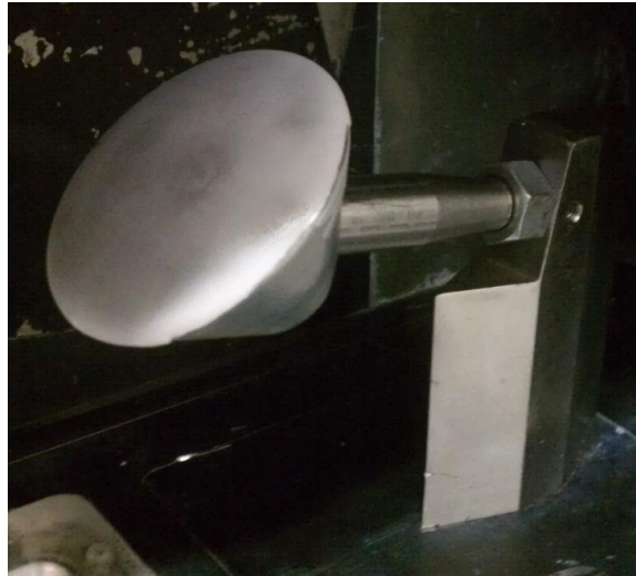
Figure 5.1: Orion MPCV model at 52° angle of attack configuration with naphthalene heat shield installed in the Mach 5 wind tunnel facility at The University of Texas at Austin.
