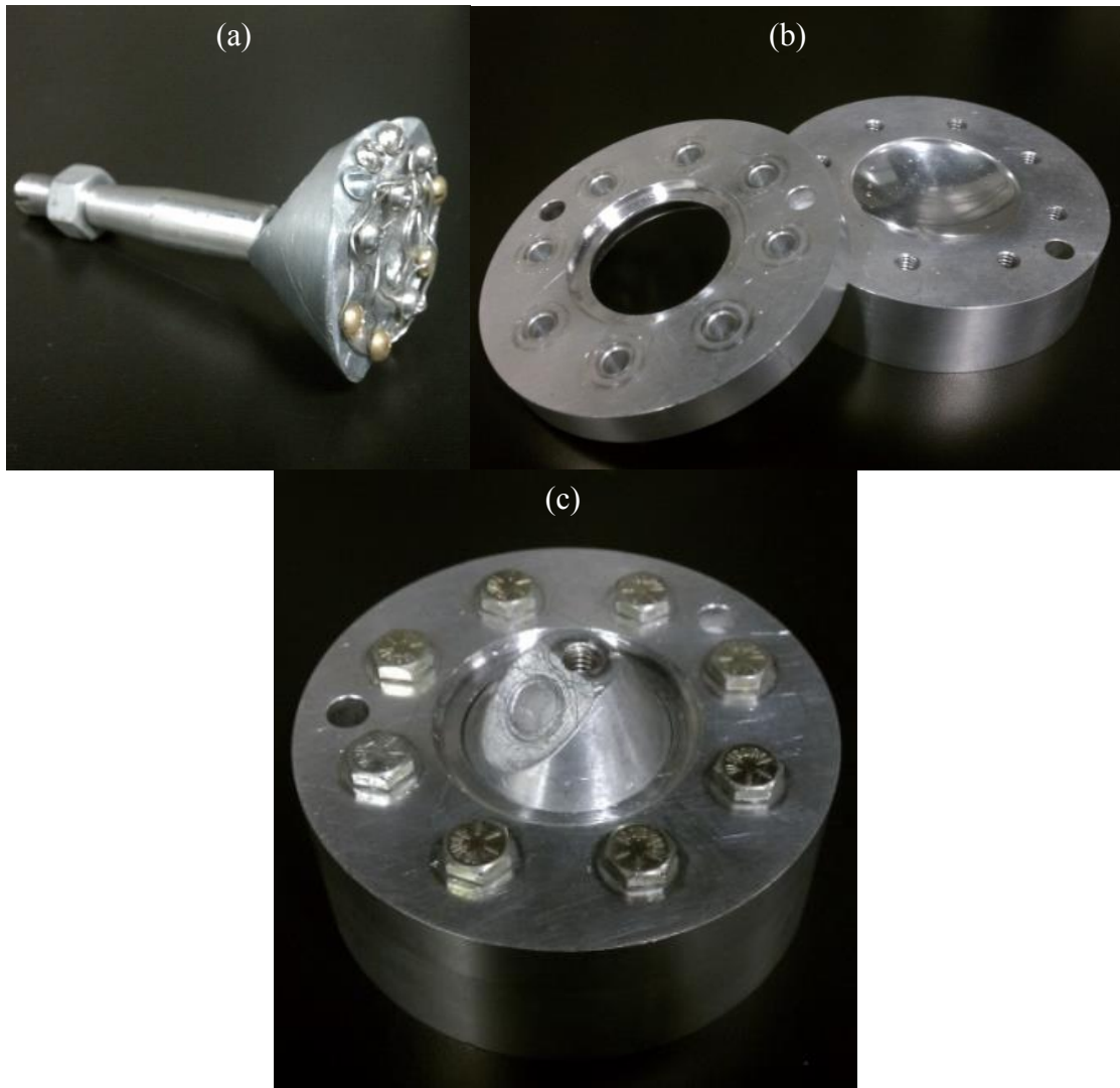
Figure C.5: (a) Orion MPCV model and sting without naphthalene heat shield, (b) top and bottom halves of mold assembly for creating naphthalene heat shield, and (c) fully-assembled mold with capsule model installed, ready for liquid naphthalene.
