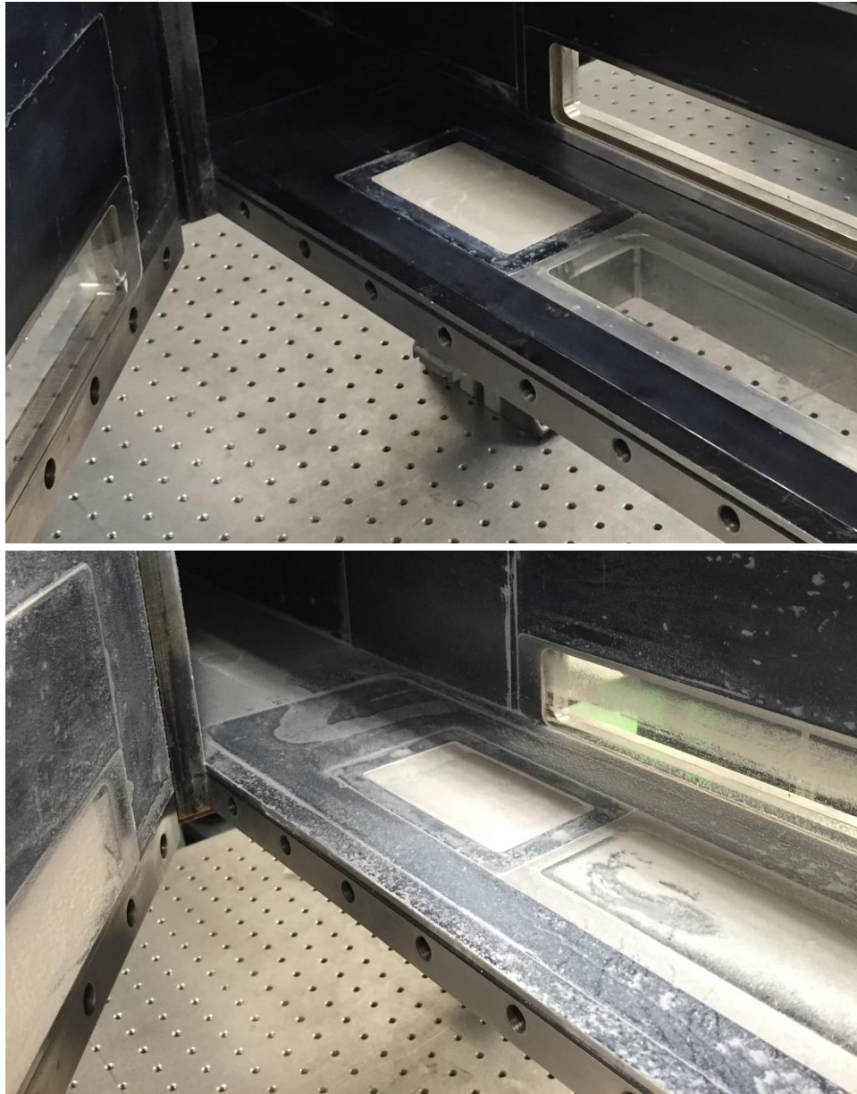
Figure 4.5: Photograph of the naphthalene insert in the Mach 5 test section before (top) and after (bottom) several wind tunnel runs with PIV particle seeding.
