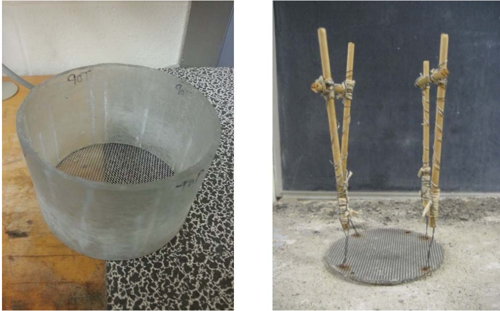
Figure 3.23: First design pluviation screen (a. left), Second design pluviation screen (b. right).
