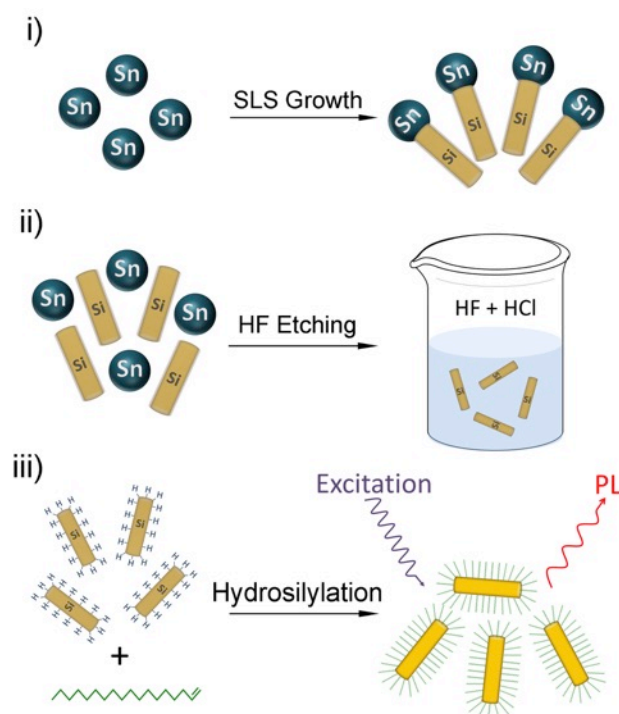
Figure 2.5 (i–iii) Illustration of photoluminescent Si nanorod preparation. (i) Si nanorods are made by Sn-seeded SLS growth. (ii) Hydride-terminated Si nanorods are obtained by HF etching in dark. (iii) Hydride-terminated Si nanorods then react with 1-octadecene to grow an alkyl monolayer via thermal hydrosilylation. The octadecene-passivated nanorods are luminescent under UV excitation.
