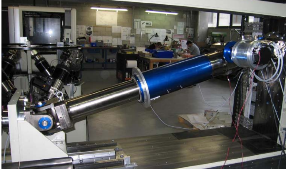
Figure 11. Test stand setup for evaluating U-joint motion
