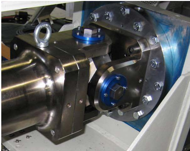
Figure 5. Actuator U-joint installed on test stand
