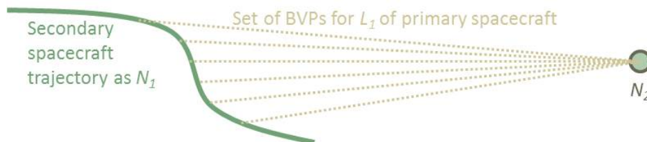
Figure 6.1: Conceptual illustration of a predefined secondary spacecraft trajectory used as a node within the MGA GS, either to deploy a primary spacecraft or as the transition from interplanetary cruise to the start of a capture sequence search.
